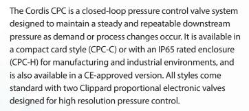
The Cordis CPC series is available with 23 different pressure sensor ranges to choose from, allowing any calibration within vacuum through 150 psig (10.3 bar) range. A 24th option—remote sensor—allows for external downstream sensor feedback. Contact Clippard for more details.
