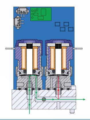
Cordis is given a setpoint command via 0-5 or 0-10 VDC, 4-20 mA, or 3.3 VDC serial
